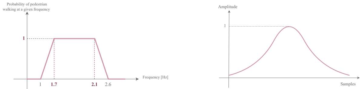
(a) Distribution of the probability of the frequency of pedestrians walking, from the SETRA guide. (b) Schematics of the shape of a Hamming window used to filter the data.
