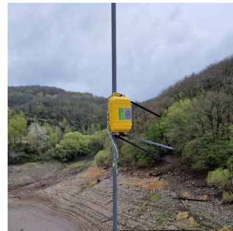
(a) G-Link-200 wireless accelerometer , used to measure the accelerations of the deck.
