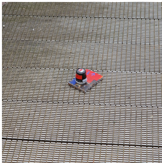
(a) G-Link-200 wireless accelerometer , used to measure the accelerations of the deck.
