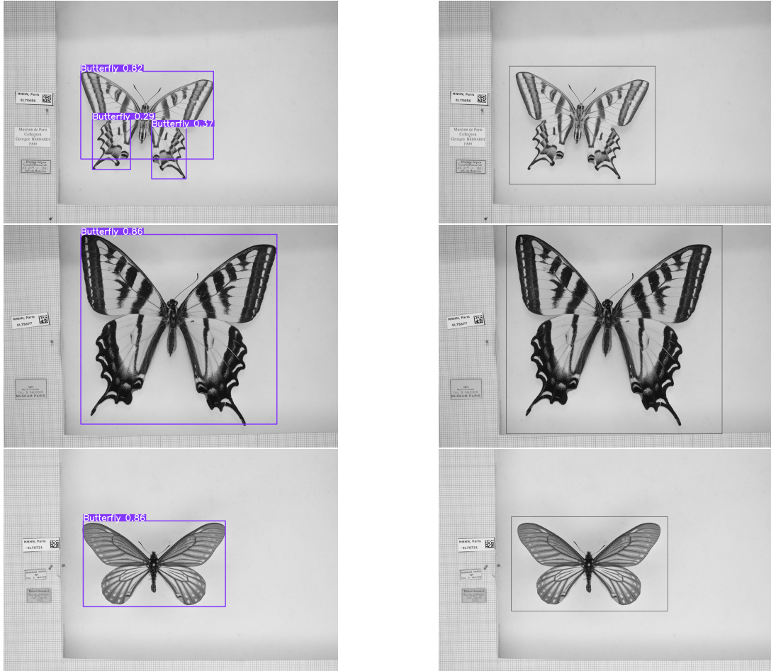
Figure 4.1: Three examples of butterfly detection and bounding box generation by a YOLOv8 model trained by Ultralytics on the "Open Image Dataset". Left column: Original images with detection boundaries overlaid. Right column: Resulting crops with 5% expanded margins. Note that the images shown are in grayscale, due to a preprocessing technique carried over from our earlier experiments with a COCO-trained YOLOv8 model that lacked butterfly-specific training.
