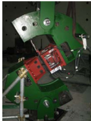
Figure 2.6: Tests on T-stub under different angles of inclination [14]
