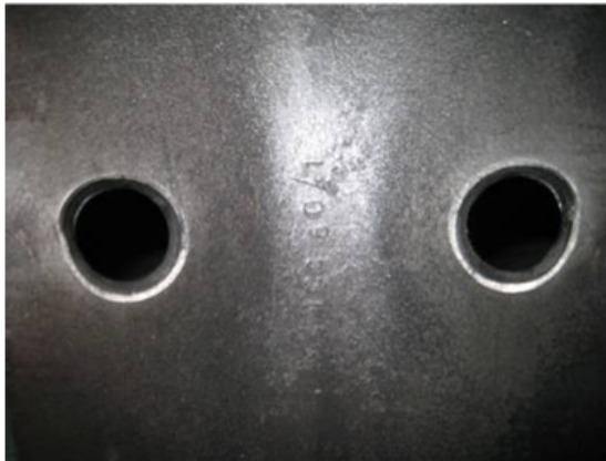
Figure 2.12: Deformation of bolt holes at collapse [3]
