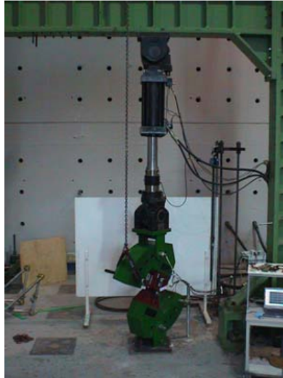
Figure 2.5: Testing apparatus for T-stub tested under axial and shear force [14]
