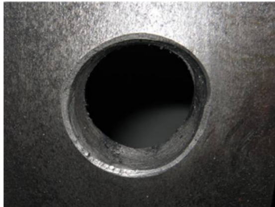
Figure 2.12: Deformation of bolt holes at collapse [3]
