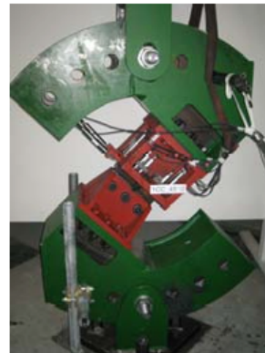
Figure 2.6: Tests on T-stub under different angles of inclination [14]
