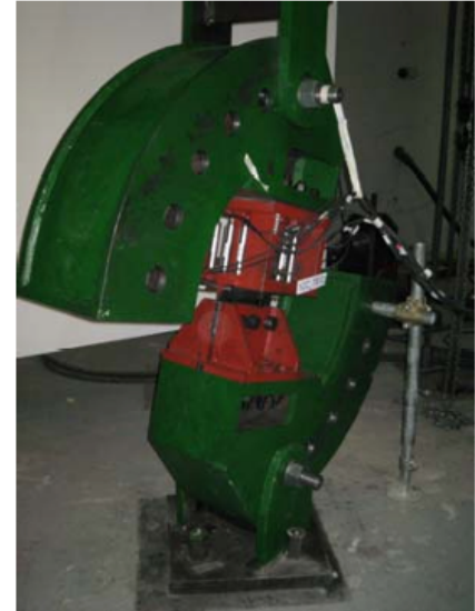
Figure 2.5: Testing apparatus for T-stub tested under axial and shear force [14]
