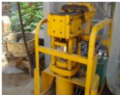
FIGURE 1.14 – Presse de compactage (Mahdad et al., 2014)
