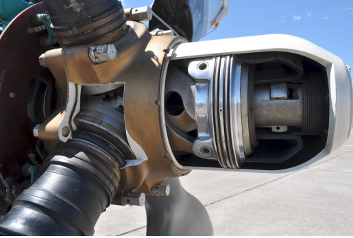
(a) C-130 Hercules variable pitch propeller[12]
