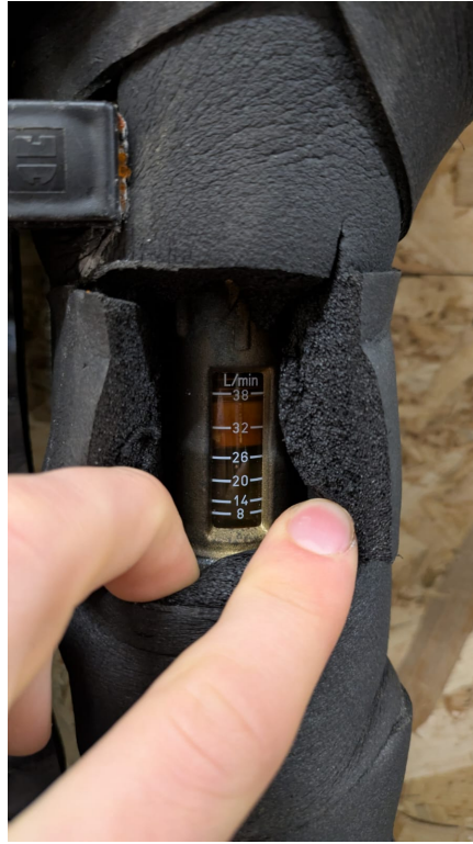
FIGURE A.9: Measured flow rate: 28.5 L/min
