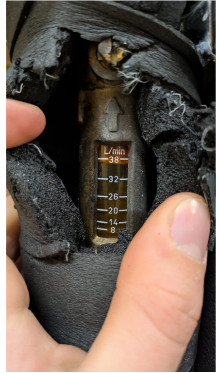
FIGURE A.10: Measured flow rate: 37 L/min
