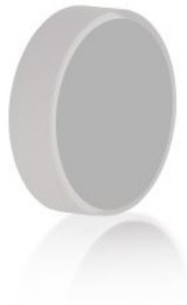
Figure 52: UV aluminum mirror 20D20AL.2, Borofloat, 50.8 mm diameter, \lambda/10 surface flatness, optimized for the 250-600 nm range, from Newport.
