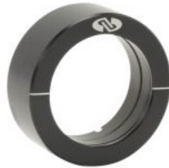
Figure 51: Achromatic half-waveplate 10RP52-1B made in Quartz-MgF 2 , 25.4 mm diameter, optimized for the range 400-700 nm, from Newport.
