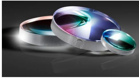
Figure 59: Converging lens #64-580, 12.7 mm diameter, effective focal length of 12.70 mm, NIR coated, molded acrylic aspheric lens, from Edmund optics.
