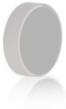
Figure 55: Dielectric mirror 10Q620BB.HR2, high reflector, 25.4 mm diameter, 0-50° angle of incidence, optimized for the range 350-1100 nm, from Newport.
