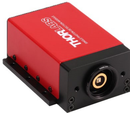
Figure 60: SPDMH2 - Single-photon detection module, optimized detection for the 400 - 1000 nm range, 100 \mu\text{m} diameter of active area, 100 hz dark count rate, from Thorlabs.
