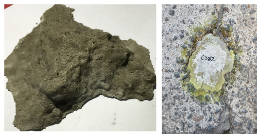
FIGURE 15 – Patch en mortier moulé (Yeon et al., 2018)
