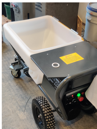
FIGURE 32 – Pompe mobile Powermat PM-AGT-3000M
