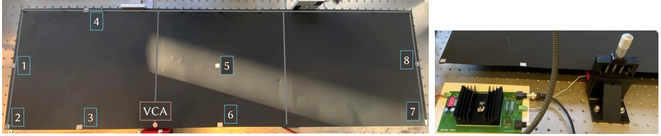
(a) Tested fin with reinforcement fork highlighted in gray, Voice Coil (b) Voice coil actuator shown on the actuator impact point shown in orange and the measurement point right with current injector at its left. shown in blue.
