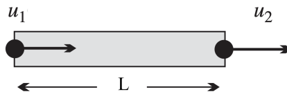
Figure 17: Bar element in 1D with nodal displacements (G  radin 2015).
