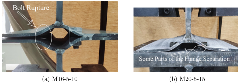
Figure 3.8: The deformation after the test [14]
