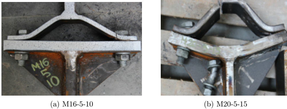
Figure 3.6: The deformation after the test [13]
