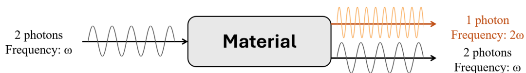
Figure 1.19: Schematic illustration of the physical principle behind second harmonic generation. On the right, the black wave corresponds to the first linear term, while the orange one corresponds to the nonlinear component, i.e. the second harmonic. To make this image, inspiration was taken from (Cantamessa, 2025) and (Tits, 2023).
