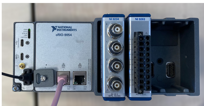
Figure 7.2: CompactRIO-9054 chassis with I/O modules (NI 9234 and NI 9263).
