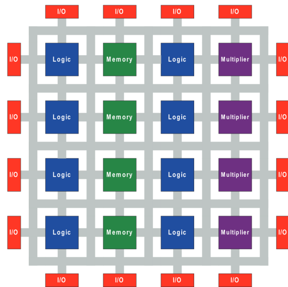
Figure 7.1: Standard FPGA architecture. [58]
