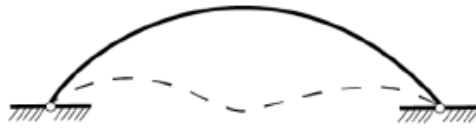
Figure 49: Snap-Through Instability Scheme - (Gens F. , Design and Construction of Bridges - Chapter 03b-1 - Arch Bridges, 2024)
