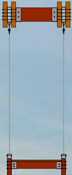
The structure is based on two curved glulam load-bearing arches, positioned laterally to the deck and connected by vertical steel hangers.
