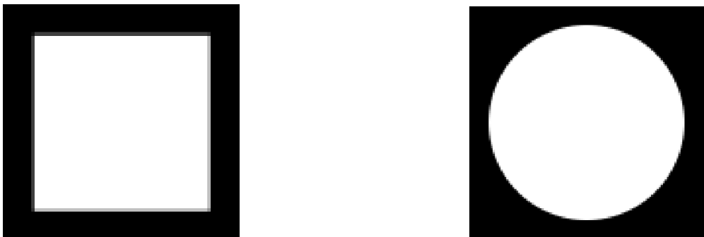
(a) Voxelized square offset by 0.75 voxel in the horizontal and vertical directions. Side length is 100 voxels. (b) Untranslated voxelized disk. Diameter length is 100 voxels.
