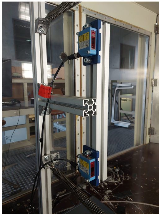
Figure 3.4: Lasers used to measure the cross-flow displacement of the cylinder.
