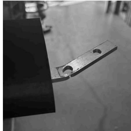
(b) Picture of the wing clamping after flutter onset was observed in ULiège experimental campaign.
