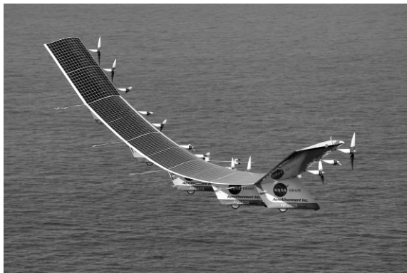
(a) Helios prototype just before breaking up.
