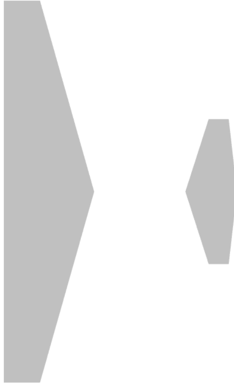
Figure 3.11: Wing and horizontal tail configuration used in the VLM analysis.
