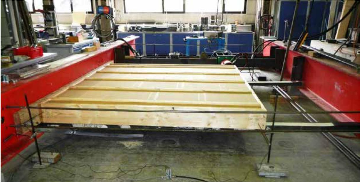
FIGURE A.7 – ILLUSTRATION DE L'ESSAI DE CONTREVENTEMENT [9]
