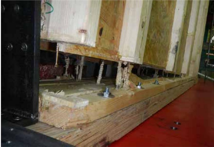
FIGURE A.11 – ILLUSTRATION DE LA RUPTURE AU CONTREVENTEMENT EN BASE DU MUR (LA TRAVERSE HORIZONTALE INFÉRIEURE S'EST DÉSOLIDARISÉE DES MONTANTS VERTICAUX) [9]
