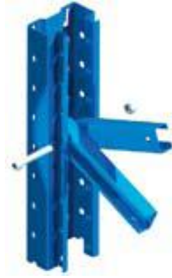
FIGURE 31 – Ames des diagonales en contact - www.stow-group.com
