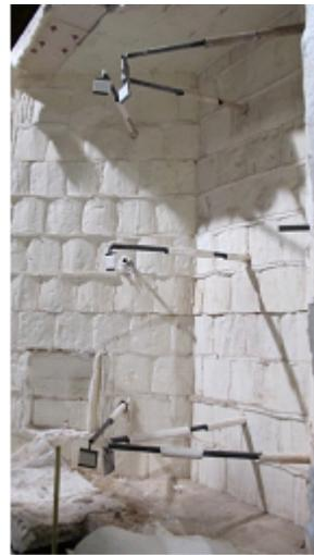
(b) 7 pyrometers located at the front side of the column through the furnace closing device
