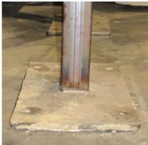
(a) Bottom end plate with holes for bolts
