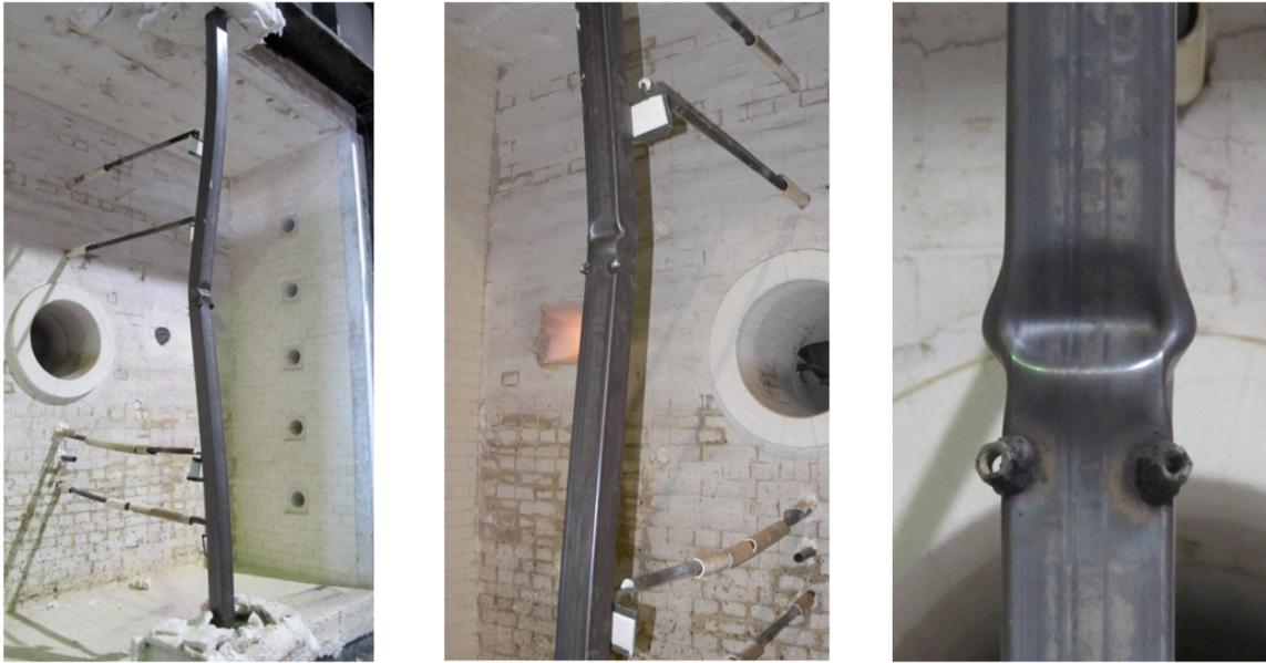
Figure 2.11: SHS 3000mm column - Failure mode
