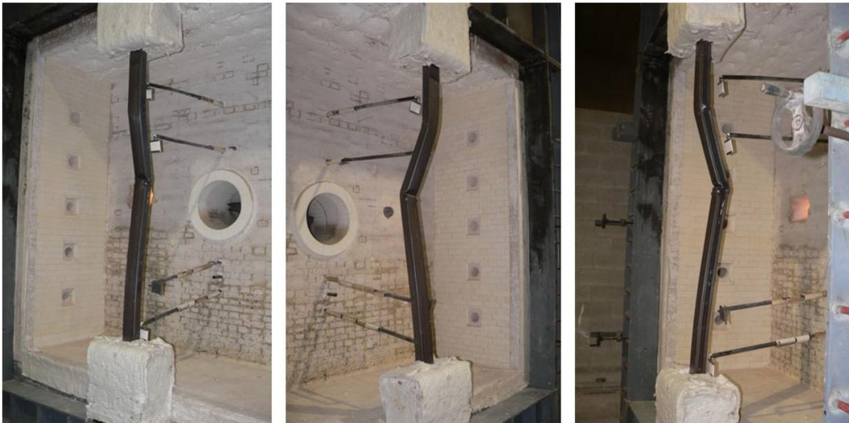
Figure 3.25: RHS 2500mm - test in fire - failure mode
