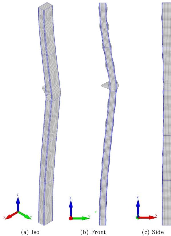
Figure 3.29: RHS 2500mm - model 8 : failure mode
