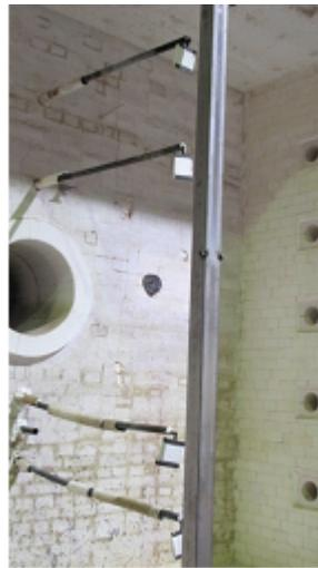
(a) 4 pyrometers located at the back side of the column
