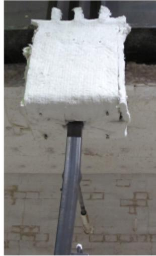
Figure 6.4: Column top end covered with ceramic fibre
