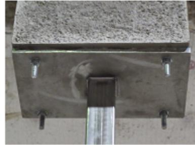
(c) Column top end with plate mounted on the concrete block
