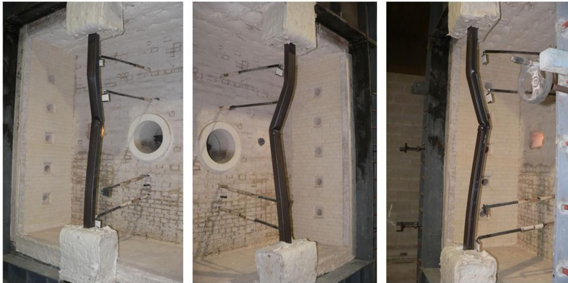
Figure 2.4: Column C3 - Failure mode
