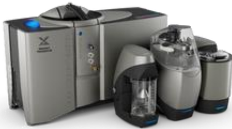
Figure IV.4: (a) Mastersizer 3000, (b) Laser granulometry principle (©Malvern Panalytical).
