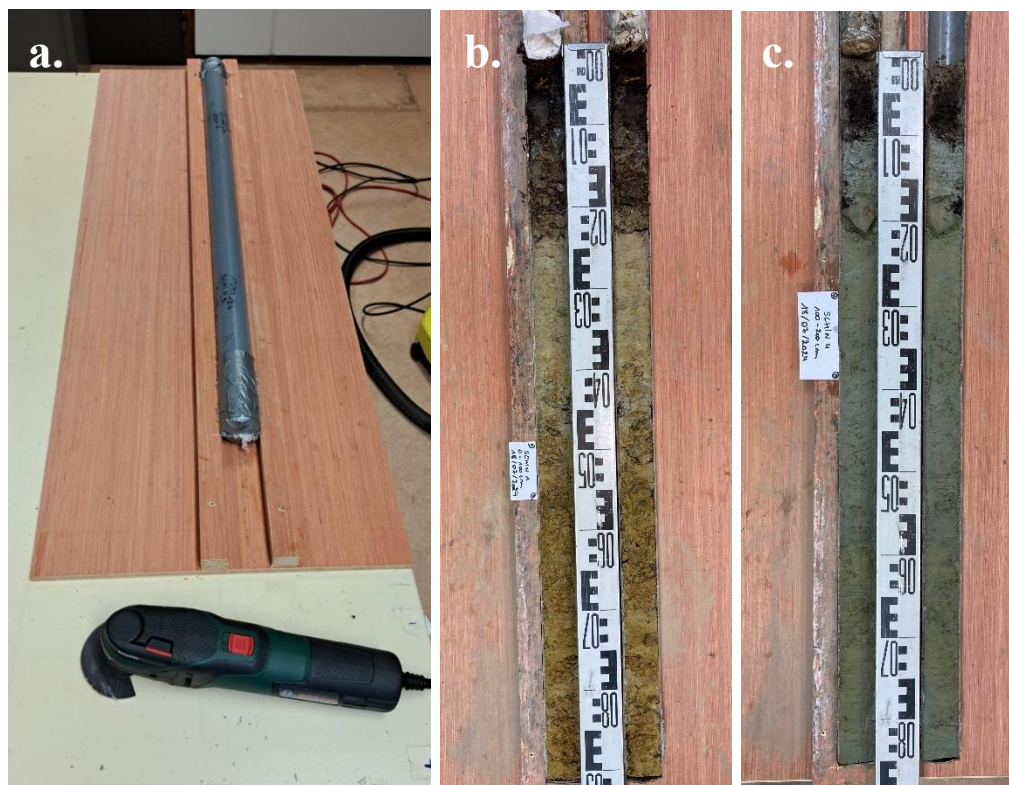
Figure IV.3: (a) Core opening equipment, (b) 0-100 cm deep core opened in two halves, (c) 10 cm thick contamination.
