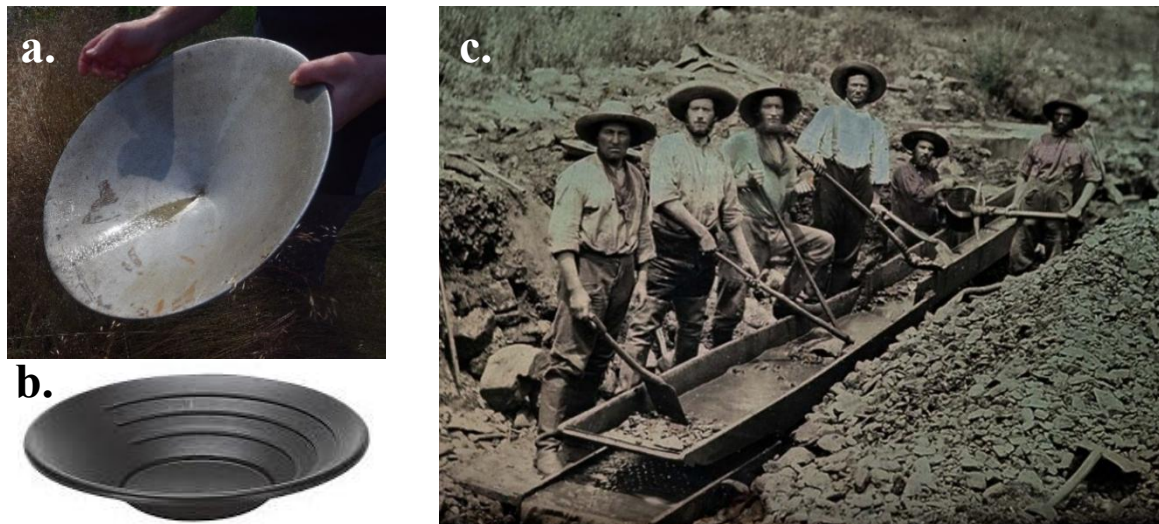
Figure I.8: Gold prospection tools: (a) batea, (b) American pan (©IRL supplies), (c) sluice box (©Western Mining History). Coarser cobbles are removed from the sluice box and piled up alongside.
