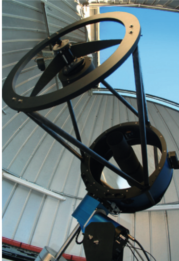
(a) Close up of the 60 cm TRAPPIST-South telescope.
