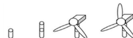
Figure 127 – Bunny ears - Assemblage de la turbine
