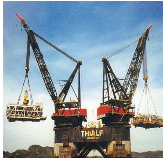
Figure 20 – Grue flottante semi-submersible 18
