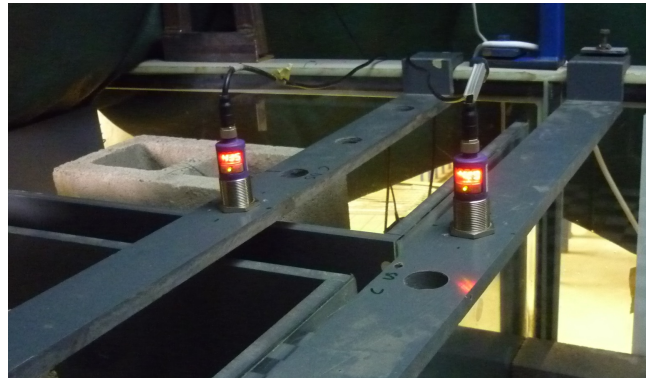
FIGURE 6 – Sketch (left) of the arrangement of the probes - The black circles represent the probes and the hatched rectangles are the supports on which they are installed - and photo (right) of the two probes located upstream of the reservoir
