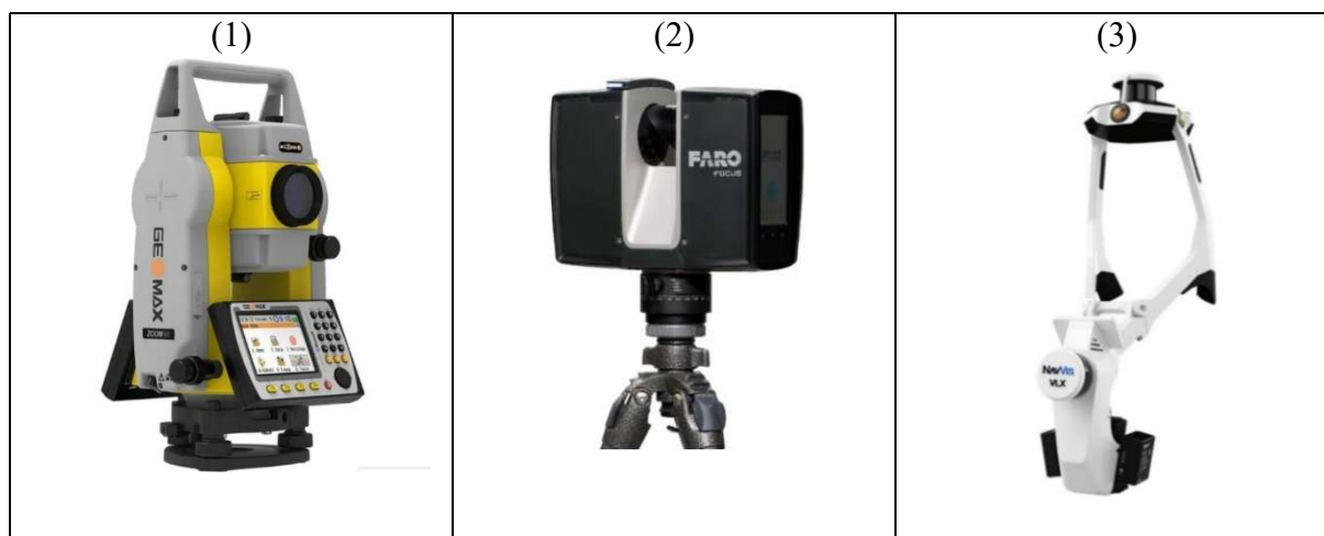
Figure 1 : Capteurs utilisés dans les techniques classiques : (1) Station totale GeoMax Zoom50 (My survey direct, 2025), (2) TLS Faro Focus premium ((Borkowski & Kubrat, 2024), (3) MLS NavVIS VLX 3 (Borkowski & Kubrat, 2024).
