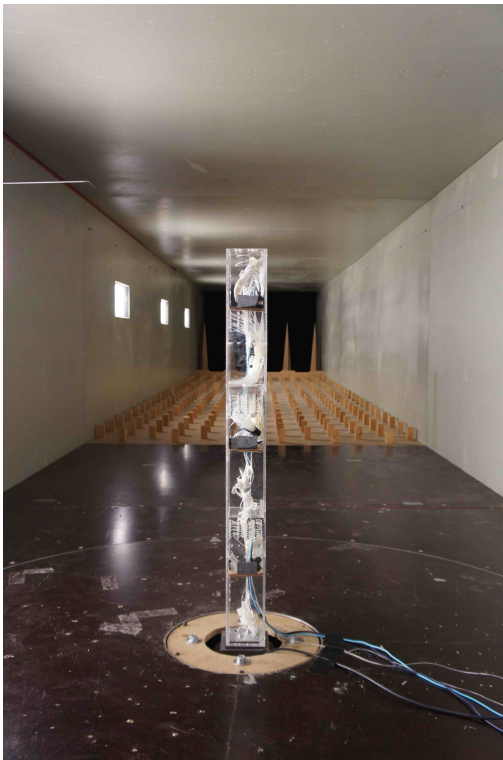
Figure 3.14 – Picture of the experimental set-up used to create the atmospheric boundary layer ABL2
