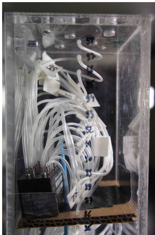
Figure 4.4 – Picture of the ESP-32HD pressure scanners connected to the plastic tubes
