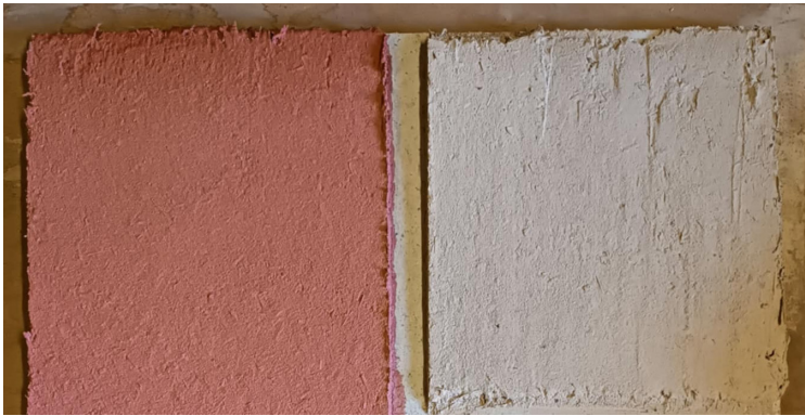
Terre, sable, chaux, fibres, colorant
