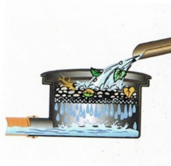
Figure 25: Fosse à sédiments (source: Vu, 2006)
