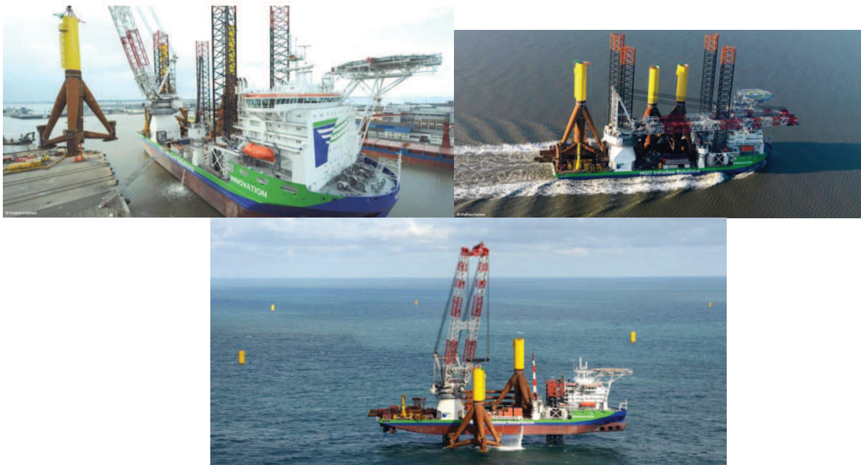
Figure 19: Tripods loading, transfer and installation
