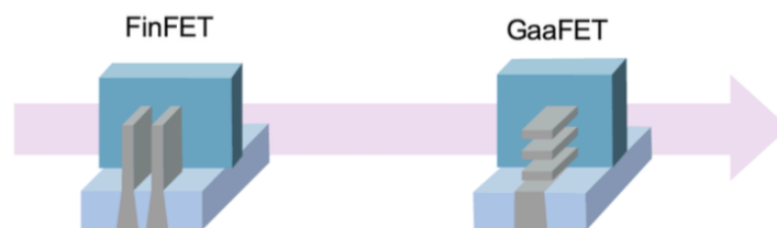
Figure 1.1: The evolution of transistor architectures from planar to FinFET and finally to Gate-All-Around (GAAFET), driven by the need for improved electrostatic control at smaller nodes. Figure extracted from [9].
