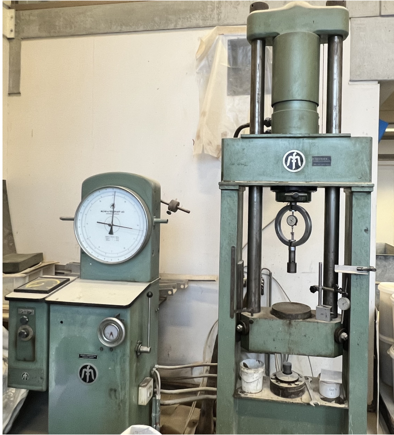
FIGURE 18 – Essai CBR standard
