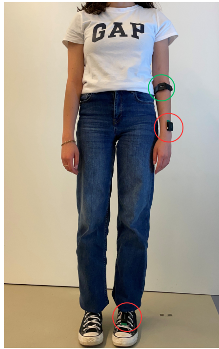
Figure 3.2: Correct sensor placements with IMUs circled in red, and the heart rate sensor in green.
