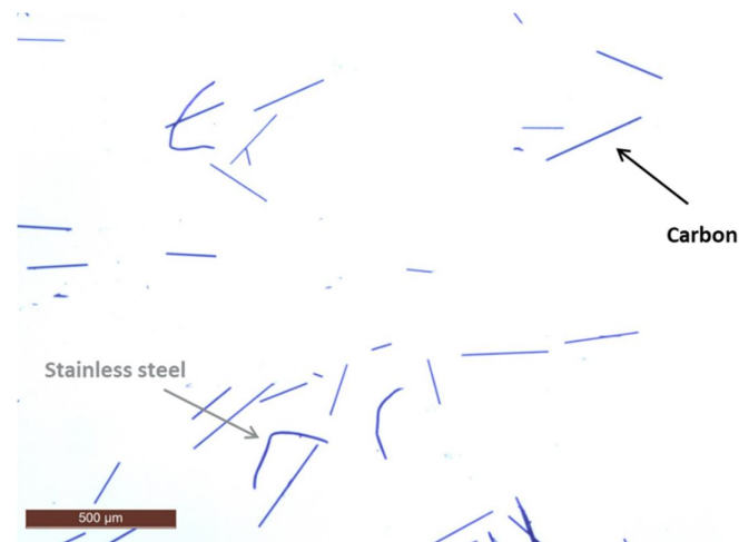
Figure 51: picture of a burnt hybrid sample obtained by optical microscopy. SF are extremely flexible (i.e. wavy shape) when compared to carbon fibers (i.e. straight line).
