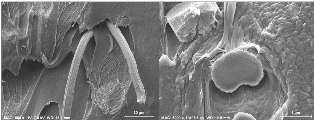
Figure 49: Stainless steel fibers fractured composite where complete fiber pull out of PA6 matrix is observed (left). PAN carbon fibers fractured composites where a fiber is still stuck into the PA6 matrix after rupture. This demonstrates a good adhesion of PAN carbon fibers (right).
