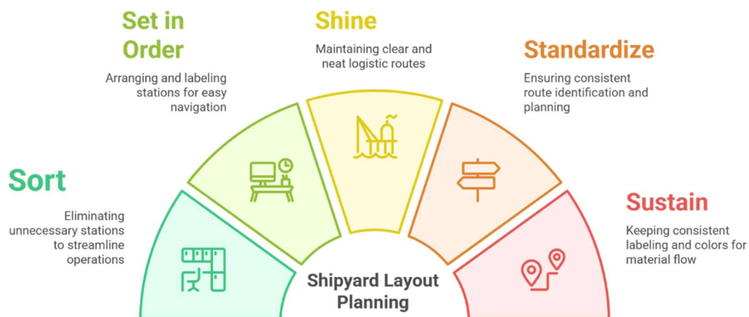
Figure 35. 5S Visual Management for Production Logistics (Generated by Napkin.AI)
