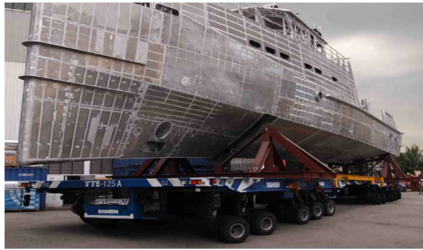
Figure 6. Movable Rack on Ship Section Transporter ( https://syncrolift.com/ )
