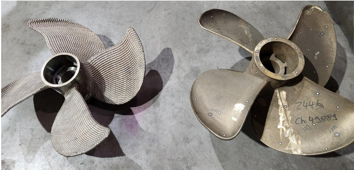
Figure 51 Comparison of 3D printed and casted propeller
