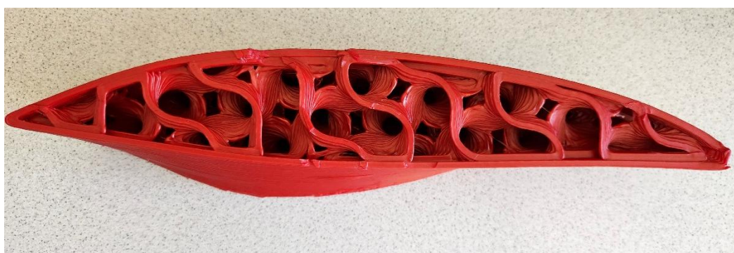
Figure 54 Scaled prototype of propeller section with gyroid structure
