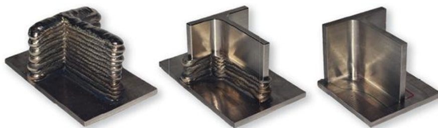
Figure 8 Hybrid Manufacturing (WAAM combined with the Milling process) (source: unconfirmed)
