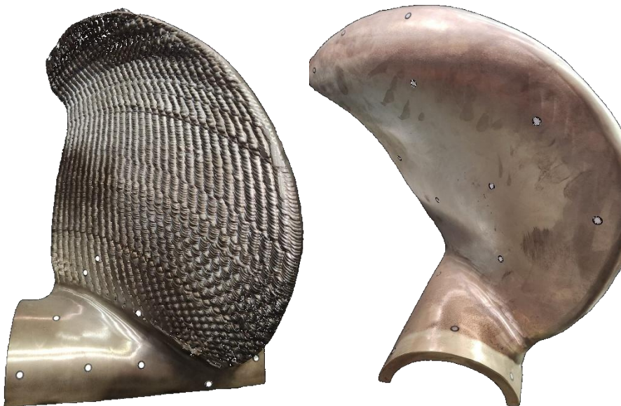
Figure 52 3D -printed Propeller with one side milled.
