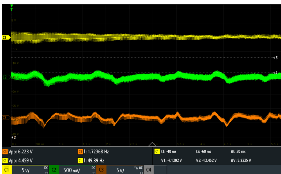
Figure 2.15: Breadboard intermediate measurements using non contact electrode
