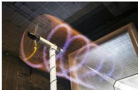
Figure 3.1 – Typical helicoidal flow create at the blade tip, behind a Wind Turbine (Mexico rotor of MexNext project), from [9]
