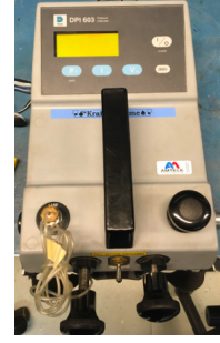
Figure 2.56 – Druck@DPI063 static calibrator in KTH, 100 [Pa] accuracy
