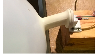
Figure A.17 – Picture of the complete setup (design 2) with 3D printed support, flush mounted transducer and PVC tube inside the balloon
