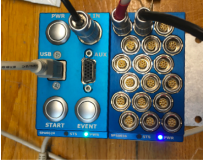
Figure 2.55 – Acquisition system Slice Pro USB controller DTS@SPU0020, Slice Pro SIM DTS@SPS0036
