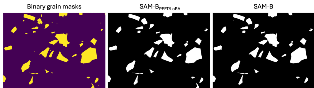
Figure 38: Full-field segmentation improvement achieved through SAM fine-tuning. Ground-truth binary grain masks (left), SAM-B PEFT/LoRA (middle), and native SAM-B (right).
