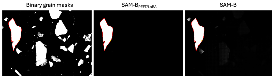
Figure 37: Mask-level improvement achieved through SAM fine-tuning. Ground-truth binary grain mask and prompted single mask indicated in red (left), SAM-B PEFT/LoRA (middle), and native SAM-B (right).
