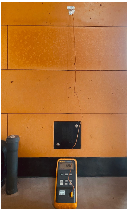
(a) Type-K thermocouple probe installation.
