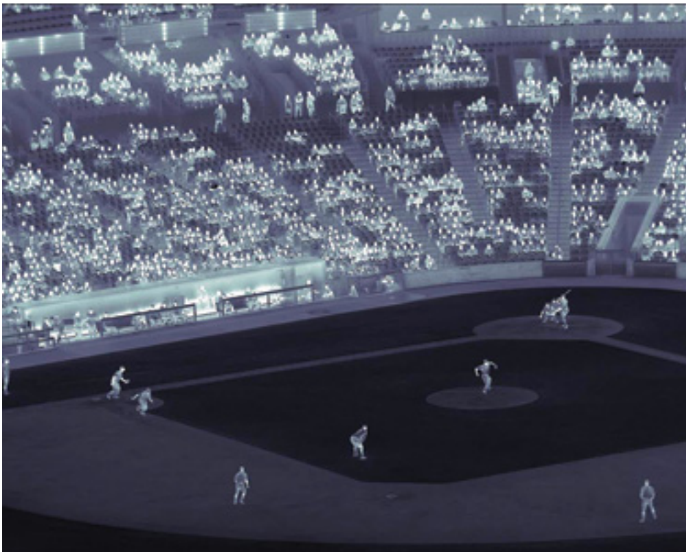
Figure 1: A mid-wave IR nBn focal-plane array (FPA) with 1280 \times 1024 pixels images a scene from a baseball game, with a player attempting to steal second base. From: Arn Adams and Elliott Rittenberg: "Advances in detectors: HOT IR sensors improve IR camera size, weight, and power", Laser Focus World, January 7th 2014
