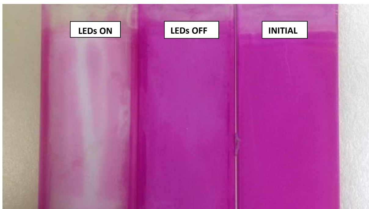
Figure 51. Comparison of the aspect of glass slides with the effect of the LEDs
