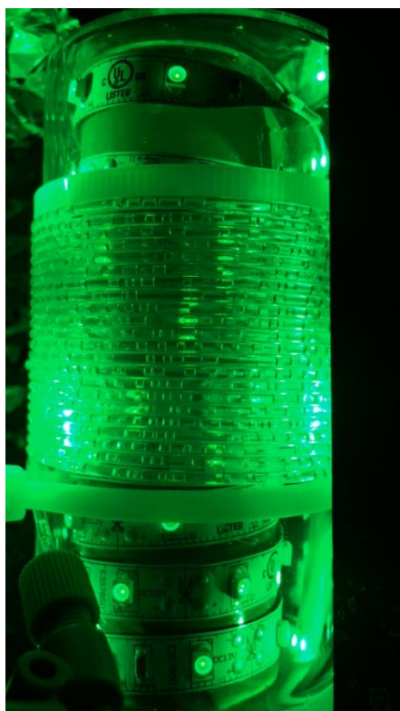
Figure 9. Microreactor system used: 4m long and composed of a 800 \mu\text{m} diameter tubing (PFA)
