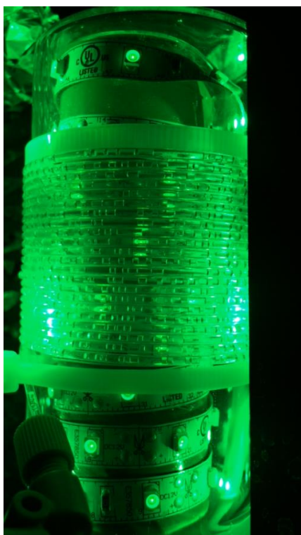
Figure 8. Microreactor system used: 4m long and composed of a 800 \mu m diameter tubing (PFA)
