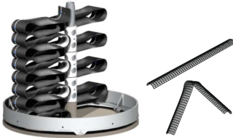
Figure 14: Stowed configuration of a tape-spring boom
