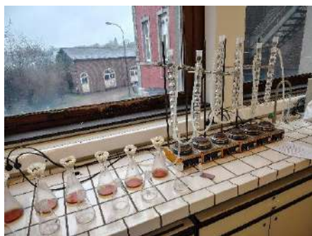
Figure 34: Extraction de matières grasses au Soxhlet (b)
