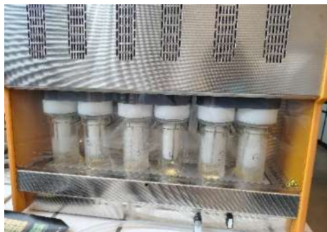
Figure 34: Extraction de matières grasses au Soxhlet (a)
