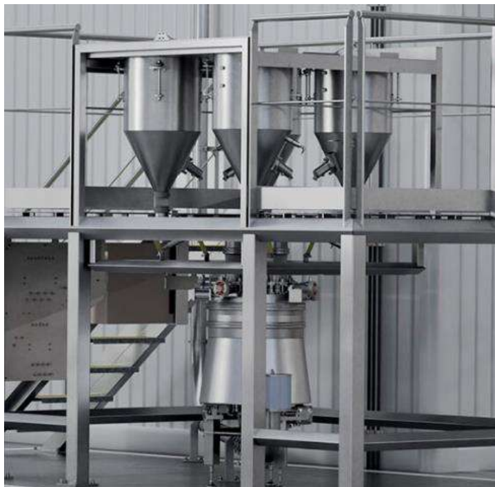
Figure 52: Station de dosage des micro ingrédients Gashor
