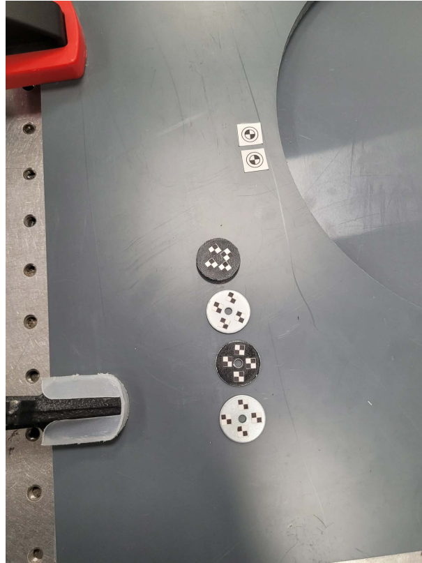
Figure 52: Photograph of the different internal masses used as NES during the experiments.
