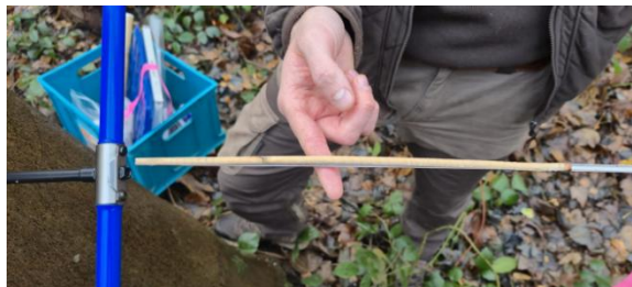
Figure 20-Tree sampling using a Pressler increment borer (Author)
