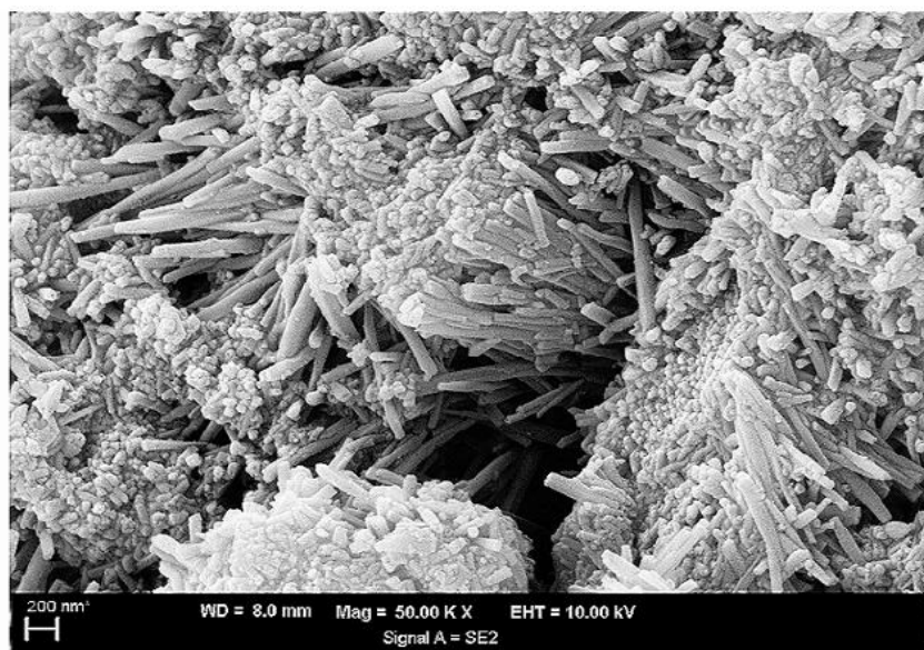
Figure 12: Tubular structure of halloysite clay [41]
