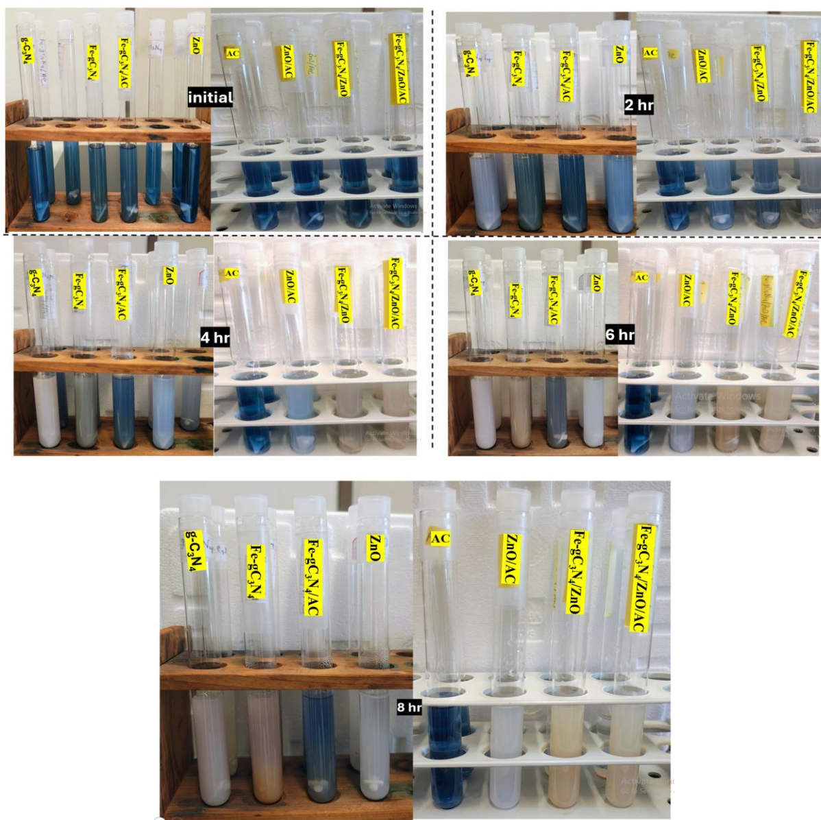
Figure 56: Visual observations of degradation of azo dye RB5 at definite time interval
