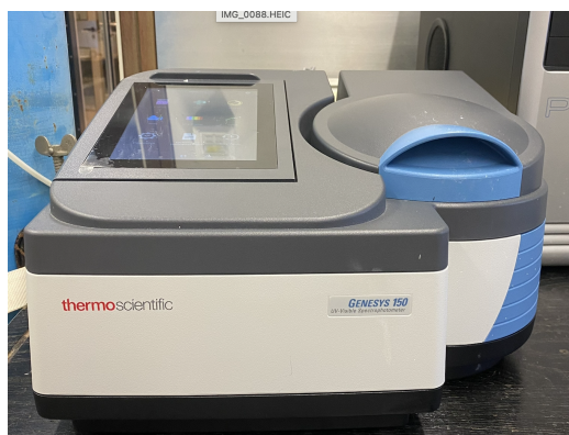
Figure 2.4: GENESYS 150 UV-visible spectrophotometer used for the experiments.
